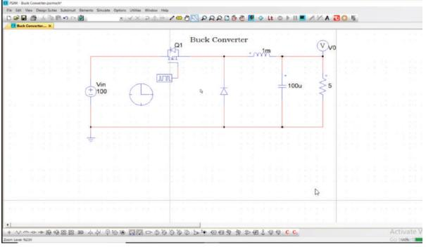
Photo: Hands on Virtual Training for Buck Converter Simulation UsingPSIM Software
