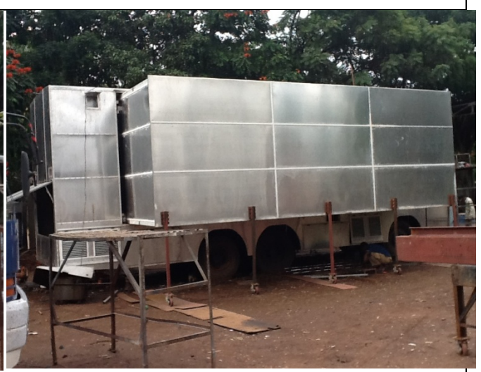
Various Stages of Fabrication of Expandable Auditorium on Wheels built on Truck Chassis
