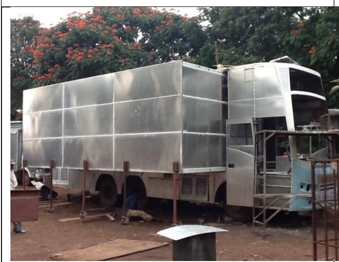
Various Stages of Fabrication of Expandable Auditorium on Wheels built on Truck Chassis
