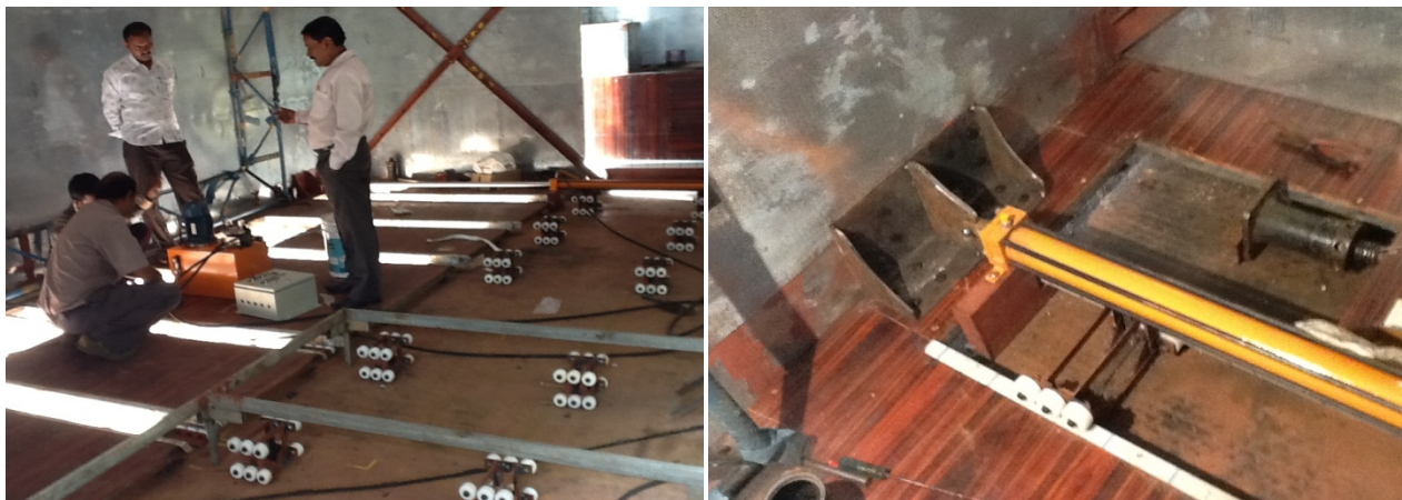
Figure 1a. Hydraulic Cylinders with Power Pack (Left) and Piston Mounting to Push Expanding Portion along with array of Teflon Wheels up & down to hold the bottom platform intack during sliding in/out (Right)
