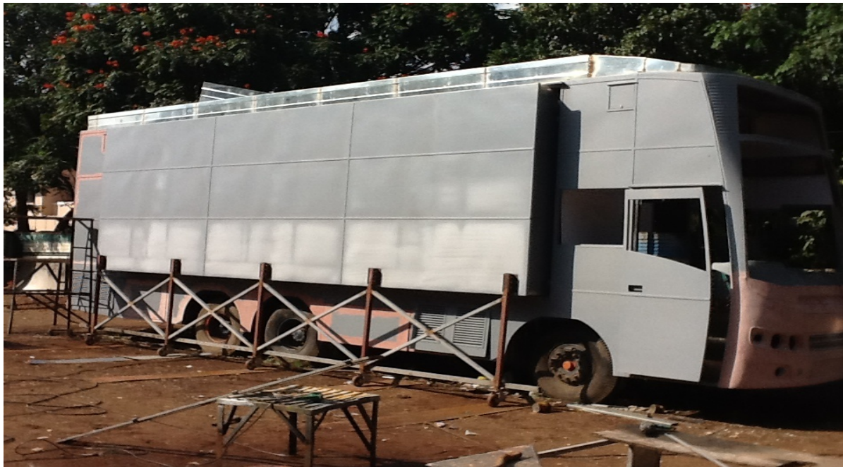
Figure 2a Five landing wheels which were assembled/attached to the outside body of expandable portion before the expansion is moving outward during expansion
