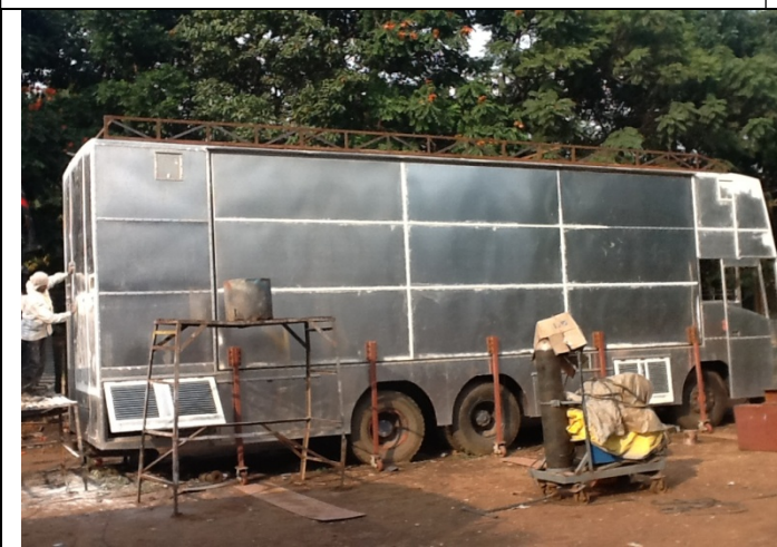
Various Stages of Fabrication of Expandable Auditorium on Wheels built on Truck Chassis
