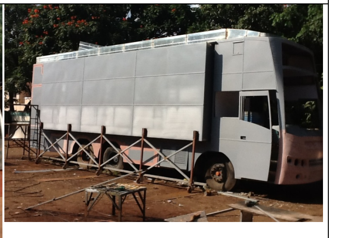
Various Stages of Fabrication of Expandable Auditorium on Wheels built on Truck Chassis
