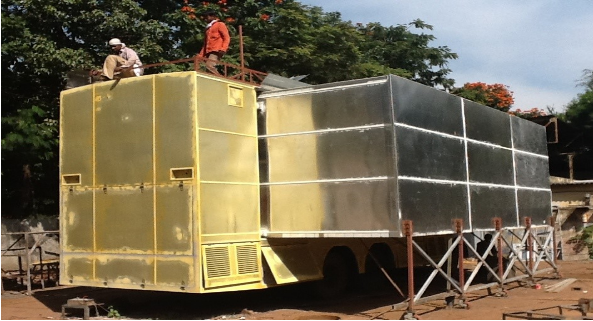
Figure 3 Fully Expanded Auditorium on Five landing wheels (Major Guiding Wheels are partly seen at Top & Bottom)
