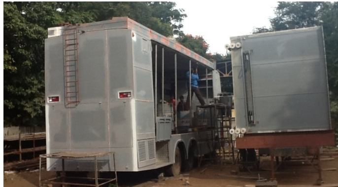
Figure 3 Fully Expanded Auditorium on Five landing wheels (Major Guiding Wheels are partly seen at Top & Bottom)
