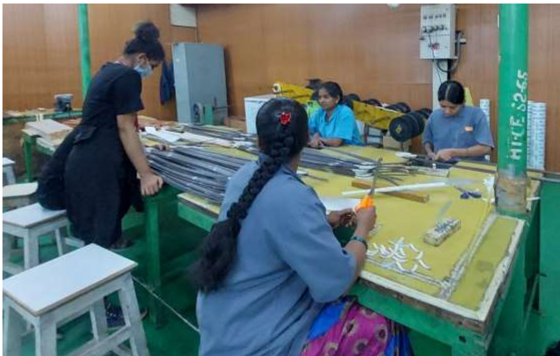
Copper coil windings being insulated by insulating papers
