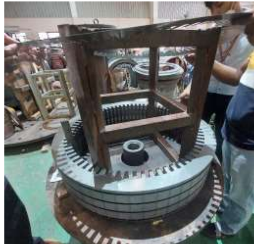
Image of stator body being assembled
