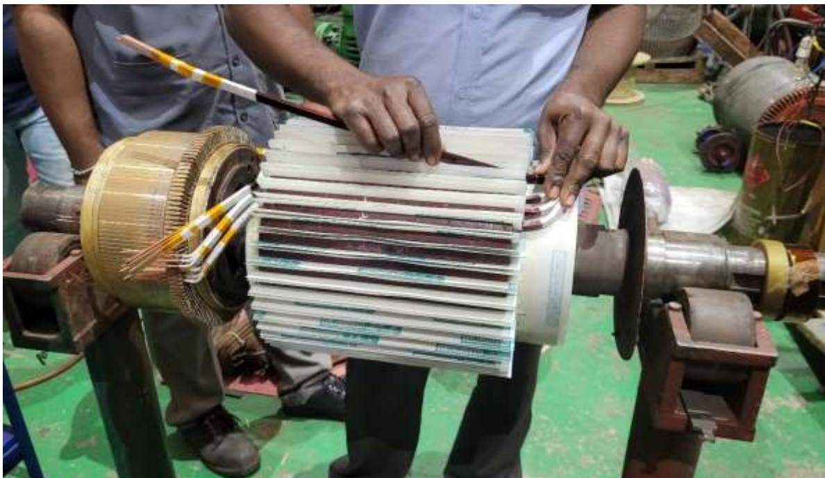
Copper coils being wound to the rotor
