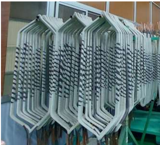
Copper coil after being shaped
